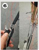
Put the orange LCL line (pic.1) through the loop on the profile and pull it tight. Repeat this step up to Rib 30 (line al2).
